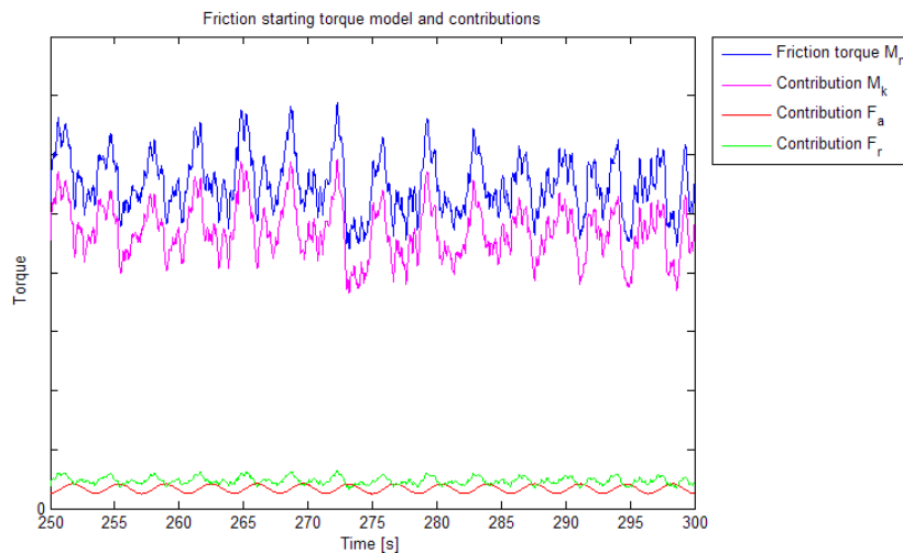
Figure 4: Friction starting torque and individual contributions of tilting moment, axial, and radial forces for 50 second interval
