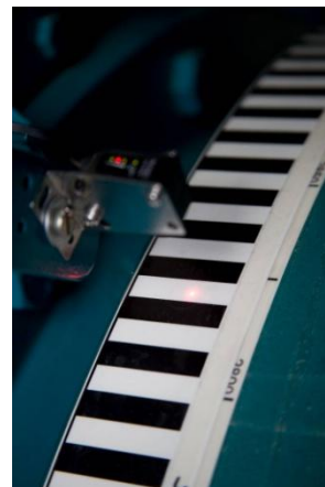
Fig. 4 Optical encoding and laser pickup for high resolved shaft speed measurements
