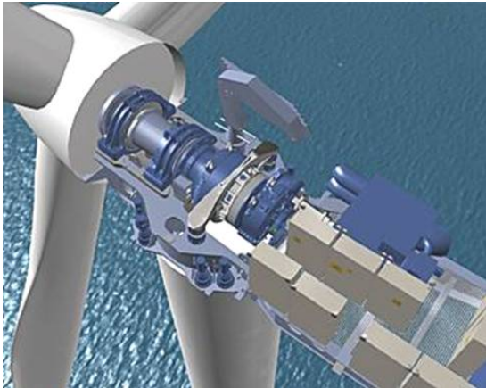
Figure 2.7: Modular drive train with two main bearings using the example of REpower 5M (Source REpower)
